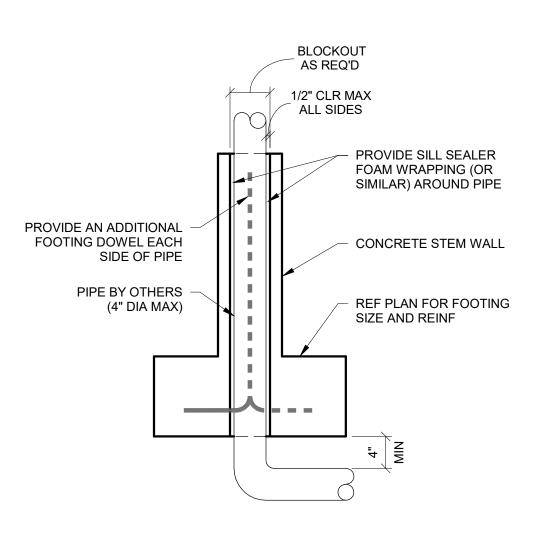
10 FOOTING BLOCKOUT AT PLUMBING PENETRATION \$501 1" = 1'-0"
