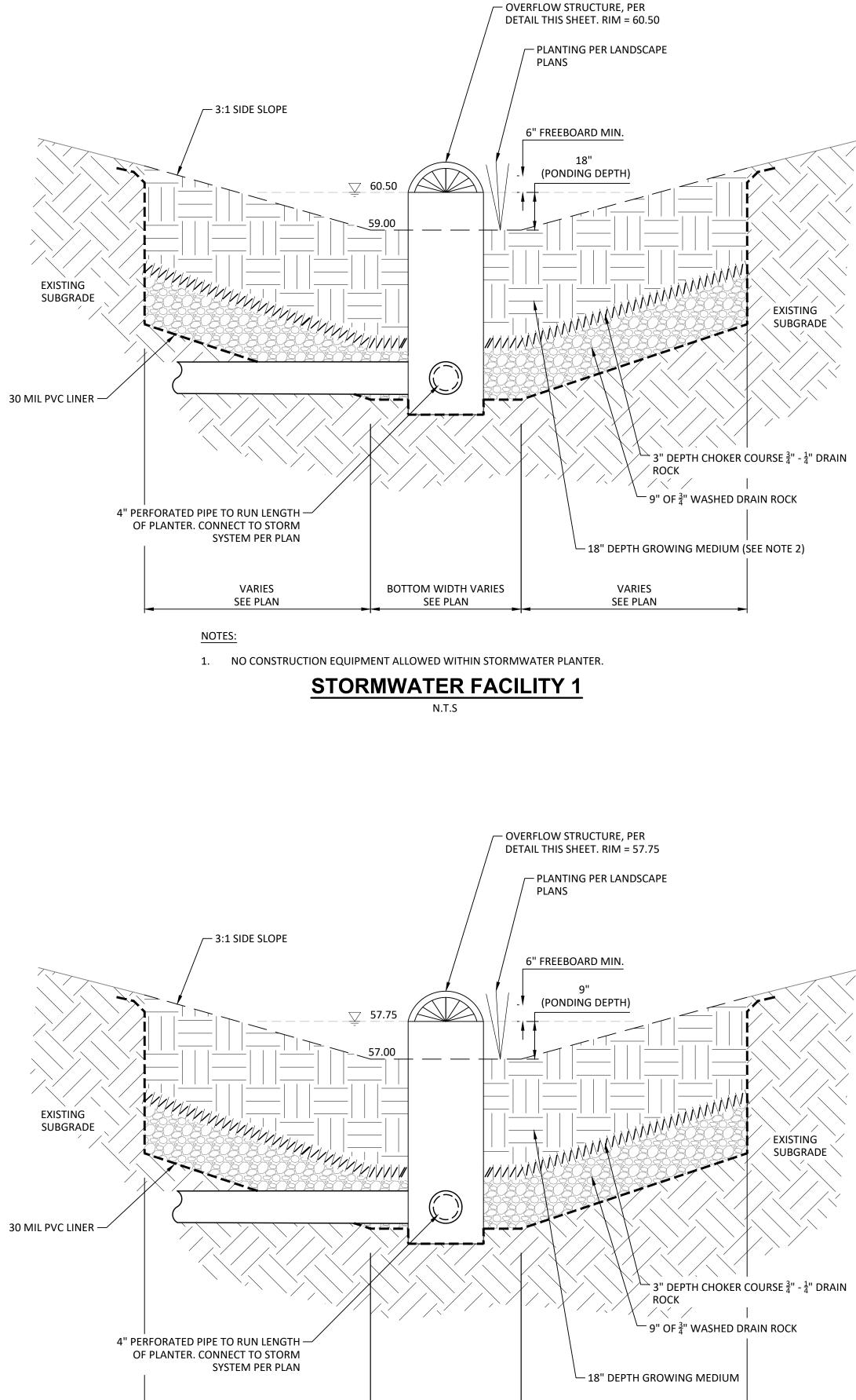
1. NO CONSTRUCTION EQUIPMENT ALLOWED WITHIN STORMWATER PLANTER.
