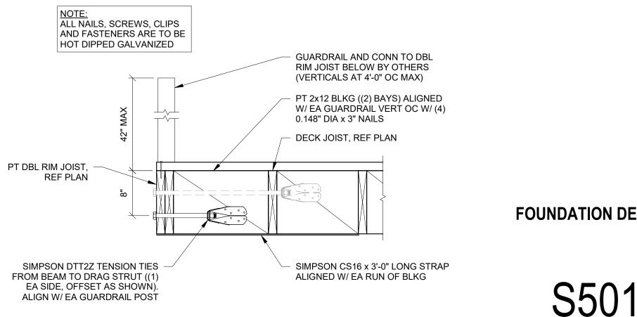
12GUARDRAIL CONNECTION TO DECK - JOISTS PARALLEL\$5011" = 1'-0"
