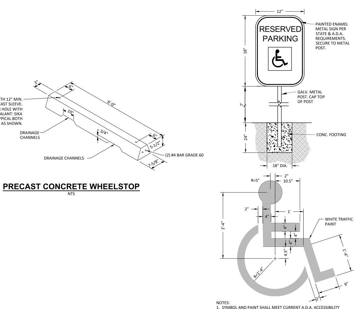
1. SYMBOL AND PAINT SHALL MEET CURRENT A.D.A. ACCESSIBILITY GUIDELINE REQUIREMENTS.
