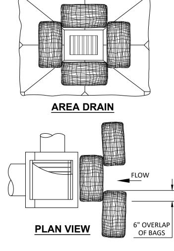
2. BIO-FILTER BAGS SHOULD BE STAKED WHERE APPLICABLE USING (2) 1"x2" WOODEN STAKES OR
