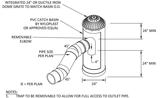
FRAMES, GRATES, HOODS, & BASE PLATES SHALL BE DUCTILE IRON PER ASTM A536 GRADE 70-50-05
